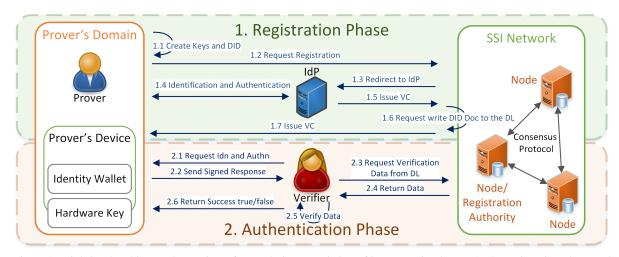
Figure 2: High-level architectural overview of our solutions consisting of its two main phases: 1. the registration phase and 2. the authentication phase.
