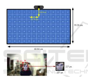
Figure 5: The data capture setup, including a sample datum. The computer monitor displays different indexed gaze locations for which the subject maintains eye contact. The camera captures a video of the subject for each gaze location. Frames are extracted, with the face then detected and cropped. With each facial image, we store the bounding box parameters (red) as well as the gaze location (yellow).
