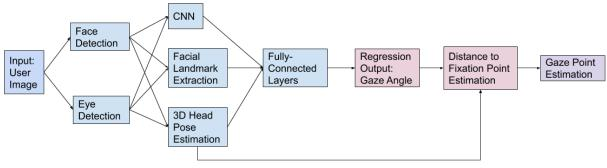
Figure 2: In previous works, a typical pipeline for regression-based gaze estimation methods may involve increased feature extractions to provide enough information to learn the complex output space. Some models discussed in the related works section estimate only up to gaze angle, while others either continue to the gaze point, or bypass the mapping from gaze angle to gaze point and instead learn end-to-end.
