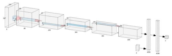
Figure 4: An illustration of one possible facial-image-based convolutional neural network block (the second stage to our system). For our experiments, we use an augmented AlexNet architure. Before the typical fully-connected layers, a 4-vector representing the position and size of the facial bounding box is concatenated to the flattened convolutional output.
