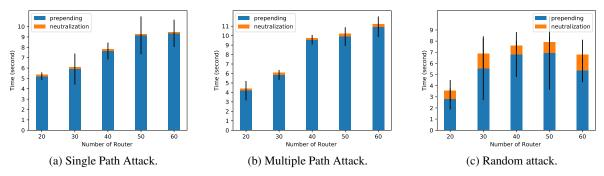
Figure 2: Resiliency evaluation results. The prepending time record increases gradually as the number of routers increases in single path and multiple path attack scenarios. While, the prepending time for random attacks fluctuates. All prepending times are presented in the form of time / 10 seconds.
