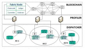
Figure 1: An overview of the three modules of BlockJack. The Blockchain module is handling data storage and data query while Profiler acts as a bridge between Blockchain and Dispatcher as well as to store the Credentials of each router. Dispatcher *monitors* routers and *dispatches* filter commands if Prefix Hijacking occurs.
