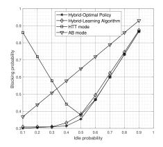
(b) The effect of the idle channel probability for  $\alpha = 0.5$ Figure 5: Blocking probability performance for different transmission modes.
