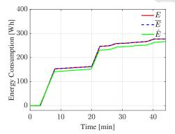
Figure 8: Comparison of the energy consumption for the QUICKWASH program.
