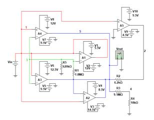
Figure 14: Evolved topology for case study 2 in complete components change mode.
