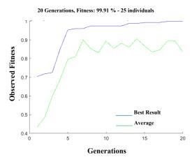
Figure 5: Best performance evolution curve for voltage divider in component addition mode.
