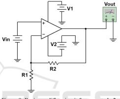
Figure 8: Basic amplifier circuit for case study 2.
