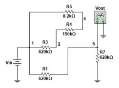
Figure 7: Evolved topology for voltage divider in full evolution mode.
