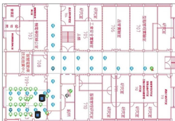
Figure 8: Experimental field plan & bNode installation location.
