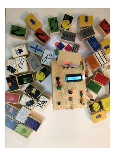
Figure 5: Kodockly 2.0 along with its programmable blocks.
