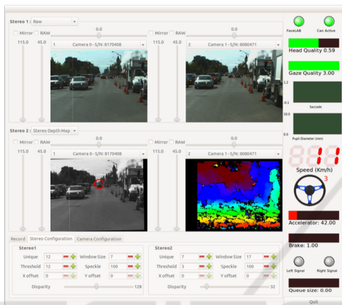
Figure 3: RoadLab software systems: The on-board system displays frame sequences with depth maps, dynamic vehicle features, and eye-tracker data.
