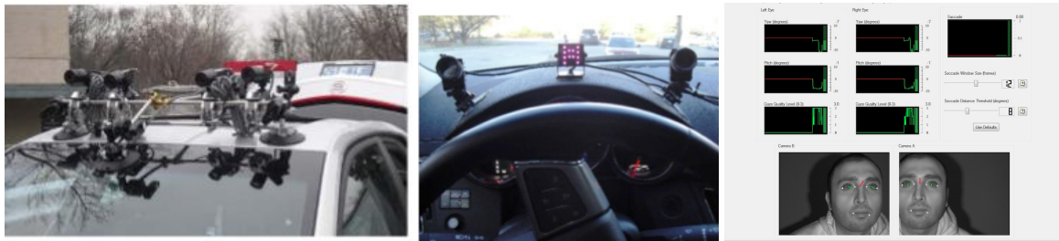
Figure 2: (left): Stereo vision system located on the vehicle’s roof; (centre): infrared gaze tracker; (right): FaceLAB system interface.
