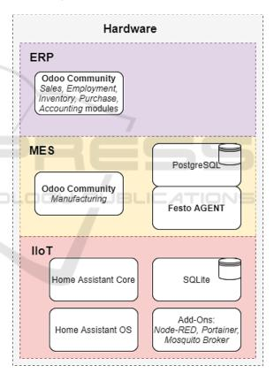
Figure 5: High Level Architecture of the enterprise software stack.
