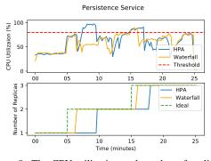
Figure 8: The CPU utilization and number of replicas for the Persistence service.
