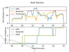
Figure 9: CPU utilization and number of replicas for Auth service.
