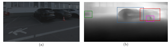
Figure 9: Input image (a) for depth estimation (b) with highlighted objects; depth encoded by increasing brightness (b).
