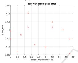
Figure 7: Error of position transducer with respect to gage blocks.
