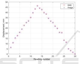
Figure 11: Displacements of target compared to that of the reference position transducer.
