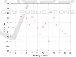
Figure 17: Error between the displacements measured from images and that of the reference position transducer.
