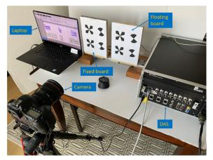
Figure 2: Front view of experimental setup.
