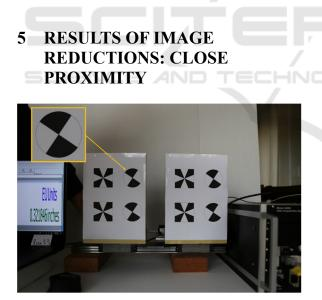
Figure 8: Step 1: find target's pattern in image.
