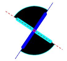
Figure 9: Step 2: Target's center as intersection of two straight lines best fit to the transition points.
