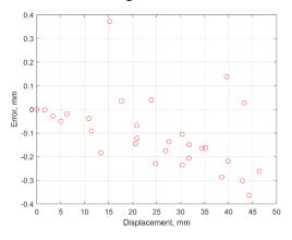
Figure 12: Error of target's center estimation with respect to the reference position transducer.
