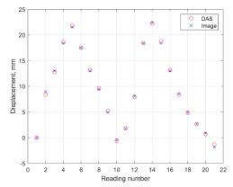
Figure 16: Comparison of the displacement measured from images to that of the reference position transducer.
