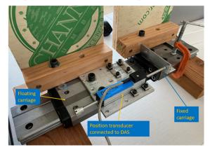
Figure 4: Reference position transducer to monitor relative displacement.
