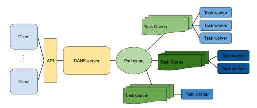
Figure 2: Schematic overview of the DANE architecture that illustrates the components that mediate the interaction between clients (the consumers of the results), and the workers (the producers of the results).
