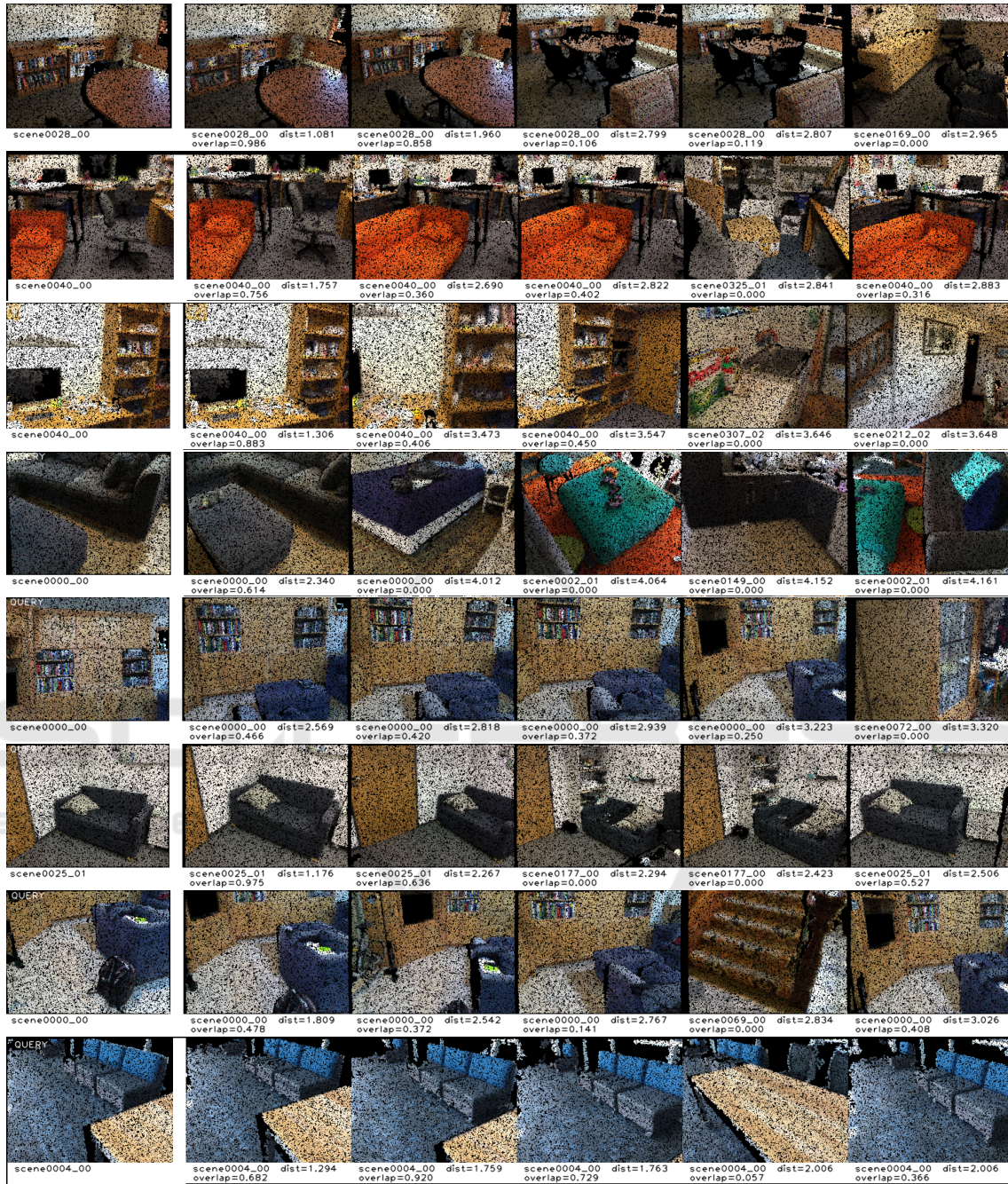
Figure 6: Visualization of point cloud retrieval results using embeddings calculated with MinkNetVLAD architecture and RGB+geometry modality. Each row shows a query RGB point cloud (on the left) and its five nearest neighbours retrieved from the database (on the right). Distance is an Euclidean distance between a query and a database point cloud embedding. Different scene names correspond to different locations.
