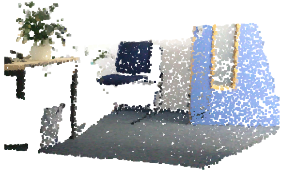
Figure 4: An exemplary point cloud generated from one RGB-D image.
