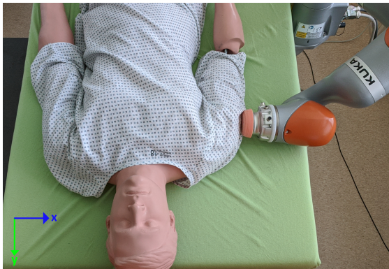
Figure 4: The setup of the robotic load experiment where the robot tries to push the 80 kg weighing patient simulator without any external help. The pushing starts at about 2.4 seconds and ends after 12.2 seconds. The torque for every joint during the execution is measured.
