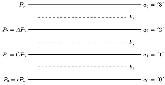
Figure 2: Representation of the ideal power levels of an optical PAM4 signal with non-zero extinction ratio and the corresponding decision thresholds.
