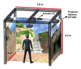
Figure 1: Schematic diagram of our KAVE Setup.
