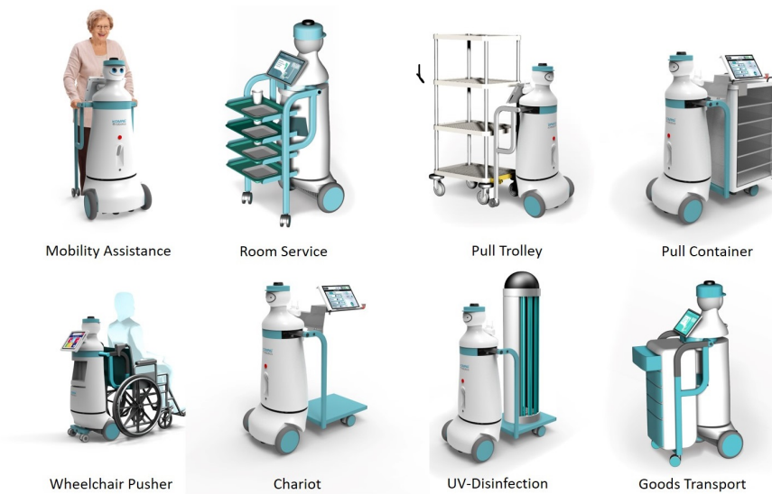
Figure 2: Overview of the different functionalities of the robots. Besides the transportation of different containers and goods, the robot can be a mobility assistance for patients or disinfect hospital wards.
