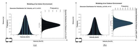
Figure 2: (a) Gaussian probability distribution functions used for modeling camera velocities and distances to features. The mean and standard deviation for an indoor environment for velocity are  $\mu = 1.3$  and  $\sigma = 0.3$  whereas mean distance and standard deviation for distance are  $\mu = 1.5$  and  $\sigma = 0.4$ ; (b) for an outdoor environment the velocity parameters are  $\mu = 3.45$  and  $\sigma = 1.0$  whereas for distance are  $\mu = 20.0$  and  $\sigma = 5.0$ .
