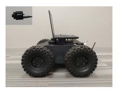
Figure 1: Dr. Robot Jaguar mobile robot platform with FLIR Blackfly S camera onboard.
