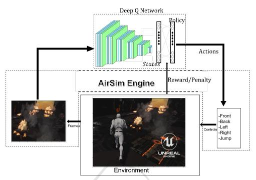
Figure 2: Architecture of Path Planning and Navigation system.
