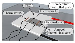
Figure 5: Scheme of experimental thermo-display and monitoring thermistors' layout.
