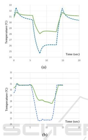
Figure 4: Comparison between simulated and reported signals - (a) Temperatures simulated at skin-display interface (green, solid) and at the display (blue, dashed), (b) Temperature measured by thermistor#2 on skin at the edge of the display (green, solid) and by thermistor #1 on the display (blue, dashed), in response to a cooling step stimulus.
