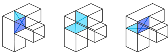
Figure 12: Three possible sets of interfaces resulting from the same geometry. The result depends on which part the intersection volume is cut out of. Since this is a random decision, the results are arbitrary. Note that the Measure of Infeasibility of the leftmost case is lower than the rest due to neither of the top parts resting on the bottom part.
