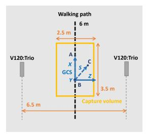
Figure 2: Top view of the setting with distance between OptiTrack bars, measures of the capture volume, length of walking path and GCS definition.
