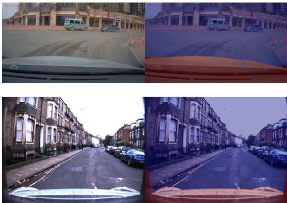
Figure 3: Masked ego-vehicle using (Arani et al., 2021). Left: Input image. Right: Segmented image with masked ego-vehicle (red) and valid region (blue). Examples from D 2 -City (top), and Oxford Robotcar (bottom) datasets. Note the varying shape, angles, and amount of ego-vehicle visibility. Only the valid region is used during feature extraction and matching for calibration.
