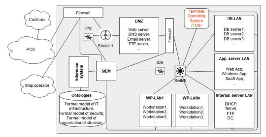
Figure 8: A high-level overview of an imaginary terminal's network.
