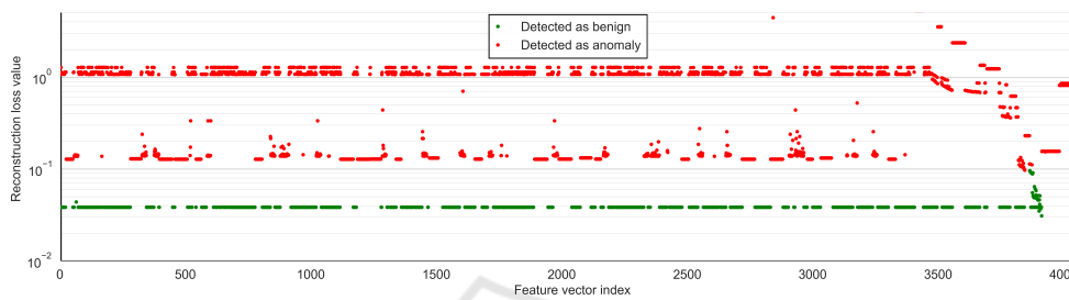
Figure 5: Reconstruction error of an AE for network data from a Slowloris attack. The reconstruction error from 1102 feature vectors are below the anomaly detection threshold and 2956 feature vectors are detected as anomaly.
