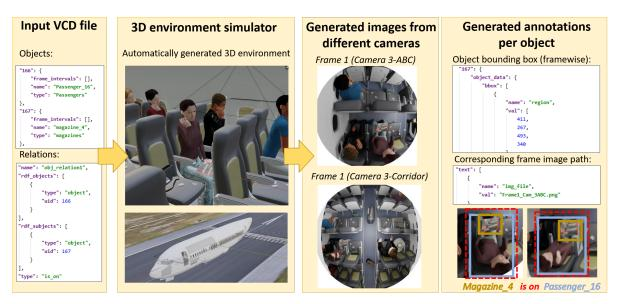
Figure 8: Data generation pipeline example. The input VCD file describes the scene that is replicated by the synthetic 3D environment generator, including present objects and its relations. The tool outputs rendered images and corresponding annotations in VCD format, which correspond to data from different camera perspectives.
