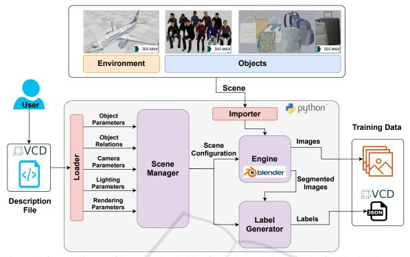
Figure 1: Software architecture of the proposed methodology for creating synthetic training data for vision-based systems.
