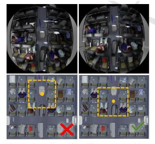
Figure 7: Captured scene from different camera positions. The configuration shown in the left images is discarded because of more occlusions.
