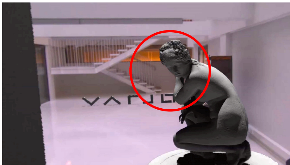
Figure 3: A still image from the left eye while rendering the test scene. For visualisation purposes a red circle for the eye direction is added. Notice the lower resolution far away from the eye direction. In addition, in the image the shadows from the virtual objects at the background can be seen at the floor and the statue is being lit also by the bounced light from the floor and the statue's stand.
