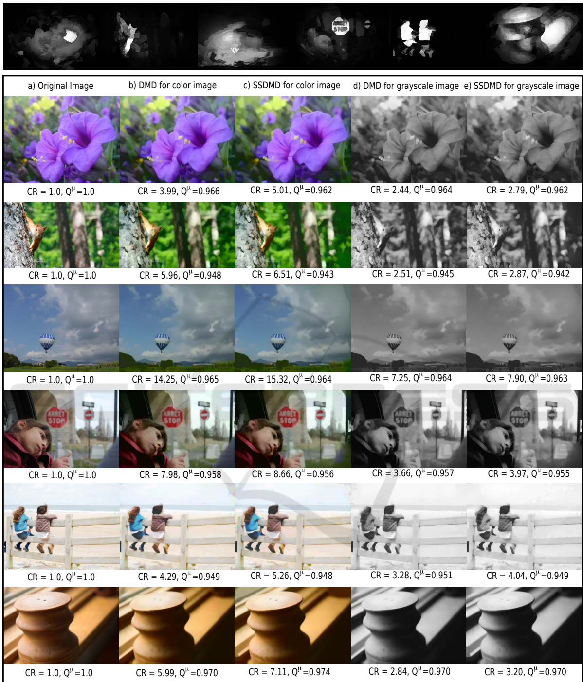
Figure 6: Comparison of the DMD with the SSDMD method for color and grayscale versions of six input images. The top row shows the spatial saliency maps of each input image. For each image, we show the compression ratio CR and quality score Q^u .
