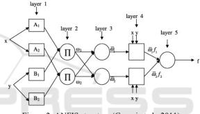
Figure 2: ANFIS structure (Guneri et al., 2011).
