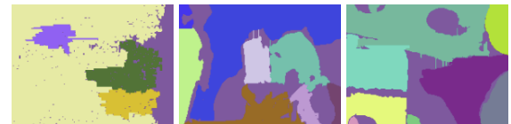
Figure 6: Our line filling approximation might result in jagged boundary artifacts in locations, where the noise is presented. The artifacts can be seen as lines that stick out of the region boundaries, as depicted in the zoomed areas of the scans.
