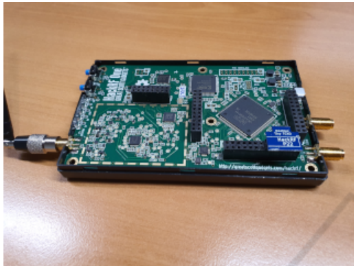
Figure 9: HackRf One with its ANT500 antenna and Tiny TCXO 10Mhz oscillator.
