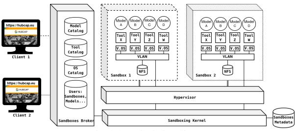
Figure 2: The HUBCAP Sandbox architecture.
