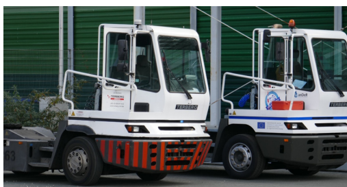
Figure 1: Diesel- and LNG-driven terminal tractors at the duisport , (Duisburger Hafen AG, 2019).
