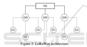
RaWAN EDs, while the NS is located near the Base Station. The Gateways could be unique and also be placed close to the BS or, in more complex scenarios where more redundancy is needed, they could be placed close to the HCs.
