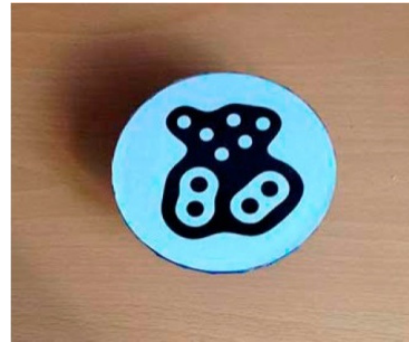
Figure 1: Example of fiducial attached to a playing piece.
