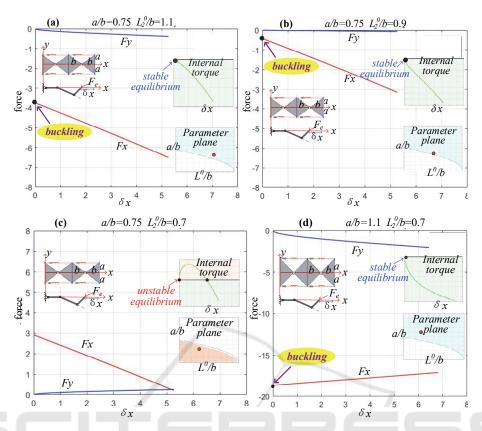
Figure 7: Force-deflection relations  $F_v(\delta_v)$ ,  $F_v(\delta_v)$  for different geometric parameters  $a,b,L^o$
