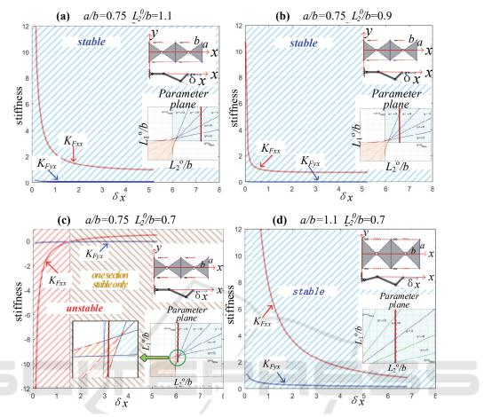
Figure 8: Stiffness coefficients for different geometric parameters ( unloaded mode ).
