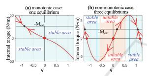
Figure 2: The torque-angle curves and equilibriums for different combinations of mechanism parameters.
