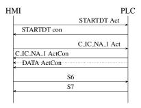
Figure 4: Sequence diagram of a Human Machine Interface (HMI) performing an General Interrogation (GI) command on a Programmable Logic Controller (PLC). The dotted line shows the injected response.
