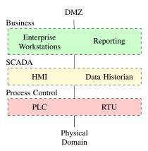
Figure 2: A high level network diagram of an Industrial Control System (ICS).
