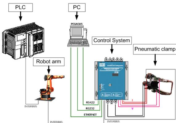
Figure 5: Experimental setup for the welding station.
