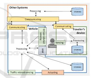
Figure 2: High level architecture of an automotive system.
