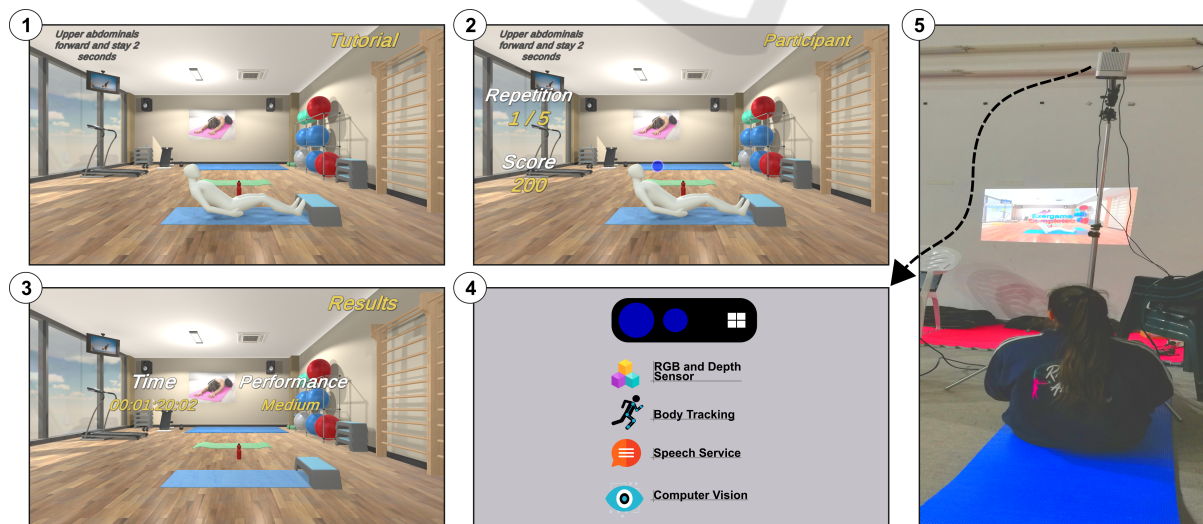
Figure 3: Rehabilitation system in action. (1) tutorial view. (2) Participation view. (3) Result view. (4) Features of the Azure Kinect DK™ device. (5) User using the system.
