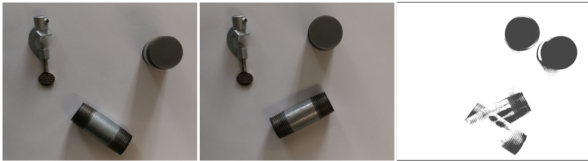
Figure 2: The image i recorded after executing a task (left), the reference image r (middle) and the calculated difference image (right). Black areas in r refer to pixel colors that deviate from each other, while white areas indicate same pixel colors.
