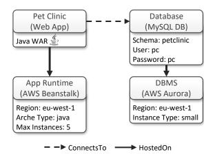
Figure 3: Simple cloud-native application expressed as EDMM-based deployment model<sup>2</sup>.
