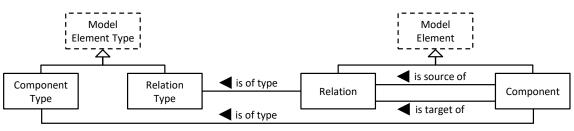
Figure 2: Simplified Essential Deployment Metamodel (EDMM).
