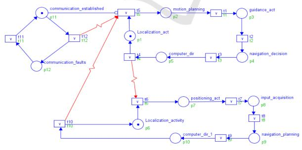
Figure 4: Dynamic Behaviour of the NCES Based-Components Model.
