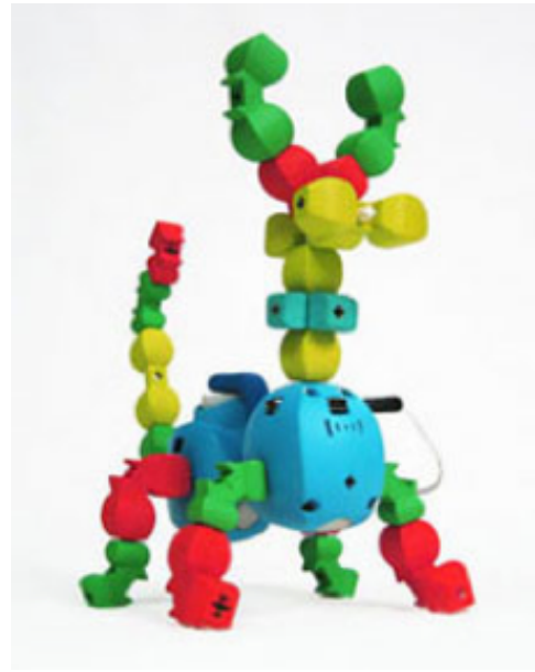
Figure 2: Topobo, a robot that can be programmed by examples. The image was taken from the official homepage (MIT Media Lab, 2003).
