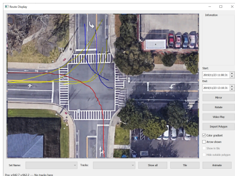
Figure 8: Collection of tracks that represent vehicles that have anomalous behavior because of their shape.
