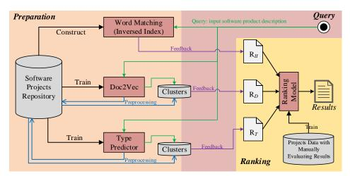
Figure 1: Framework of the proposed Software Project Searching Approach.
