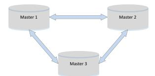
Figure 1: Cluster-based multi-master architecture for a high availability database.
