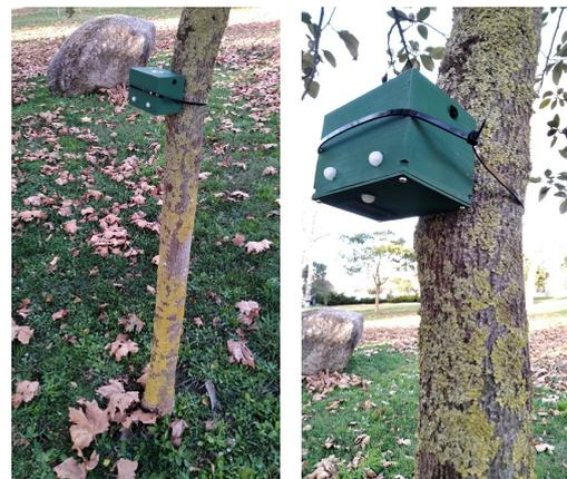
(a) Prototype fixation. (b) Placement of sensors.
